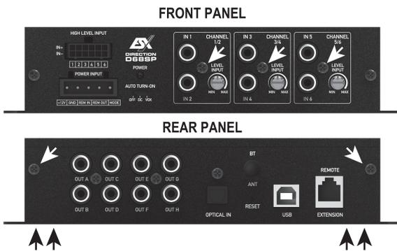
**3** Carefully pull away the upturned sheet metal part of the housing towards the front panel.
