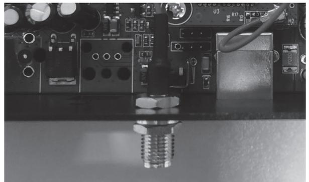
**8** The assembly of the housing is now carried out in reverse order of steps 1 to 3. Finally screw the enclosed antenna onto the SMA socket on the device.
