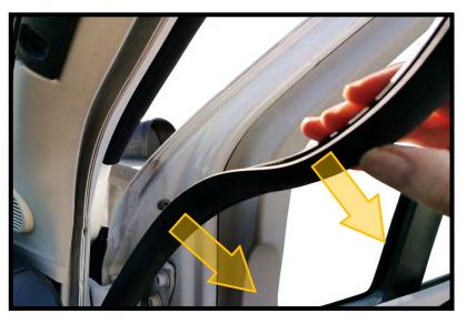
2 Remove the rubber seal from the door frame.
