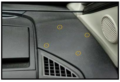
$\begin{array}{c} \textcircled{12} \\ \hline \end{array} \text{ Drill the holes with a 2.5mm drill.} \end{array}$
