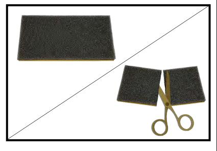
(15) Wrap one piece of the adhesive foam around the connector and stow it away behind the A-pillar trim.
