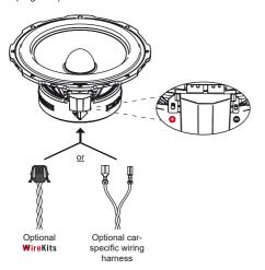
**Option b:** Universal connection via optional available CWK FX.W-550CC cable, e.g. in active applications
