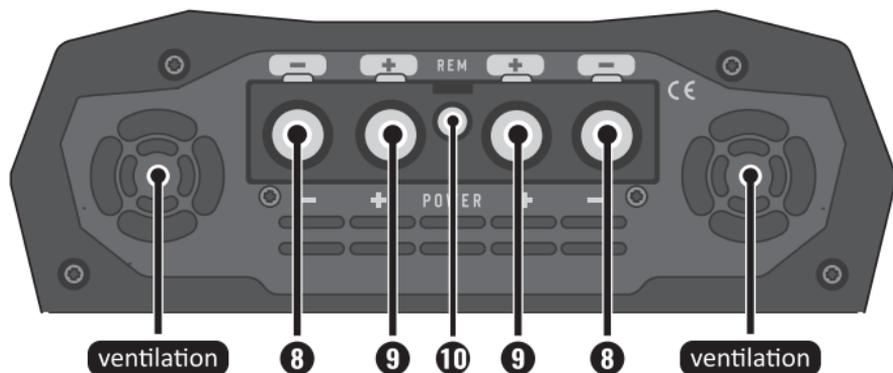
**8. DOUBLE CONNECTOR  $\ominus$  (GROUND):** Make the connection with the battery ground terminal using two cables of at least **00AWG** with up to 3 meters (one for each ground input of the amplifier).
