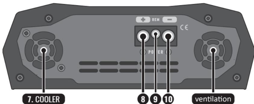
**7. COOLERS:** It cools the amplifier. Install in a cool place being careful to not obstruct the air vents.
