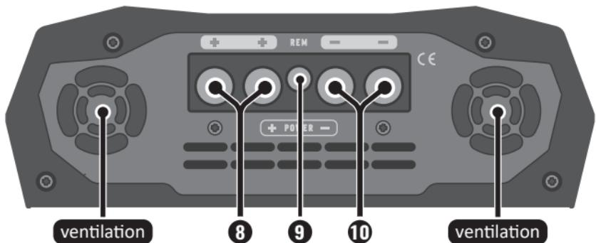
**8. POSITIVE POWER SUPPLY CONNECTOR:** Connect to the positive battery terminal of the battery using a minimum **00 AWG** cable with a fuse/circuit breaker installed as close to the battery as possible.
