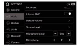
Under **Internal AMP** you can switch the device's integrated audio amplifier on or off. If you are using the device's preamp outputs to drive an external audio amplifier, turn off the amplifier.
