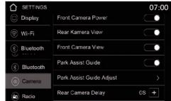
Here you can switch on the rear or front camera, switch on the respective power supply via the device and activate the respective view in the camera menu.
