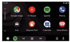
In order to use **Android Auto**, you must first connect your smartphone to the device using a USB charging cable or Bluetooth (see page 18). Bluetooth and Wi-Fi must be activated on both devices. You may still need to install the Android Auto app and activate it for this connection.
