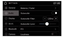
**Subwoofer** activates the SUB1/SUB2 preamp outputs. Thea cut-off frequency can be set under the **Subwoofer Filter**, i.e. all frequencies above are filtered out. Below you can adjust the **Subwoofer Level**.
