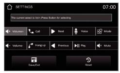
If your steering wheel remote control has been correctly connected to the device, you can teach the individual functions to the device here. As soon as you have assigned all functions, leave the menu with Save/Exit
