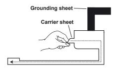
Remove the carrier sheet from the black amplifier unit and the foil antenna and stick the antenna onto the window
