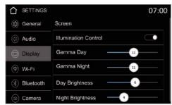
With **Illumination Control** you can activate the control function for the day and night light mode via the connected headlight signal.
