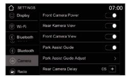
You can use the **Park Assist Guide** slider to turn on the rear view camera guidelines. With **Park Assist Guide Adjust** you can adjust the guidelines.
