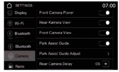
Under **Rear Camera Delay** you can set the delay in seconds with + with which the rear camera should be displayed on the monitor when engaging reverse gear.
