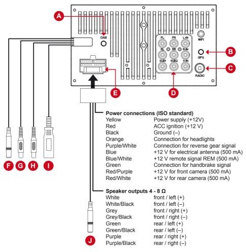
If your vehicle does not have a suitable ISO system plug, you must use the included 16-pin ISO double plug and connect the corresponding connections to the open cable ends as described above.
