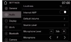
Under **Microphone** you can choose which microphone should be used for the hands-free function. **F** is the internal microphone on the control panel and **R** is the external microphone connected to the back of the device.
