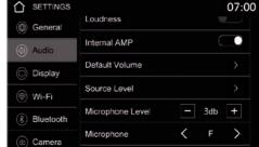
With **Default Volume** and **Source Level**, you can tune and adjust the levels for each application and signal source as desired.
