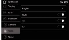
With **AF**, the radio switches to an alternative, better frequency of the station in the network if the reception signal is too weak and an alternative frequency is available.
