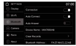
Under Auto Connect and Auto Answer you can specify whether your smartphone should be automatically connected to the device after a restart and whether calls should be answered automatically. Under Clear Records, you can delete devices that have already been registered.
