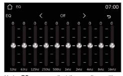
Under **EQ** you can adjust the equalizer settings manually or use the < *I* > buttons to select one of the presets. **Loudness** increases the highs and mids to make the sound louder and more powerful.
