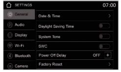
Under **Power Off Delay** you can use -I + to set the seconds for how long the device should remain switched on after the ignition has been switched off.
