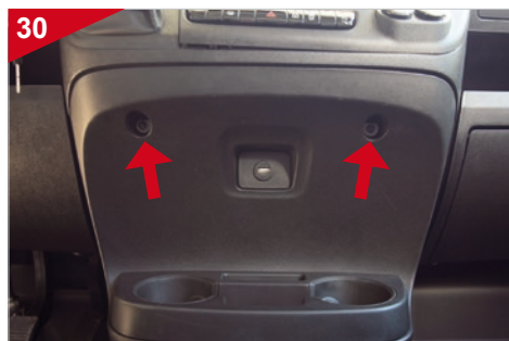
Remove the two screws from the cover on the lower center console.
