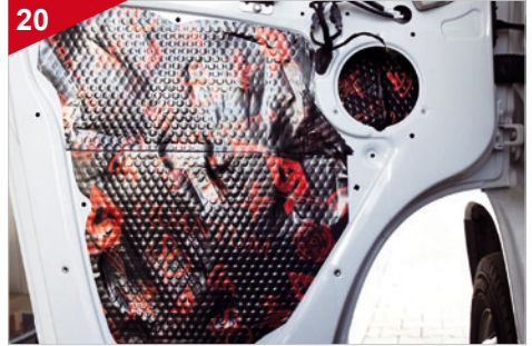
20 OPTIONAL: Then tape the entire area that was previously covered with the white foam, which you can also use as a cutting template.
