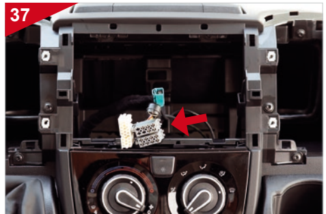
Plug the two ISO plugs into the corresponding ISO sockets (B and D) on the amplifier wiring harnesses supplied.
