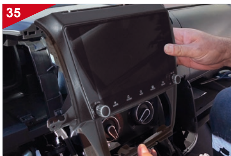
Detach the original radio or naviceiver in the dashboard. Depending on the installed device, the appropriate method varies.
