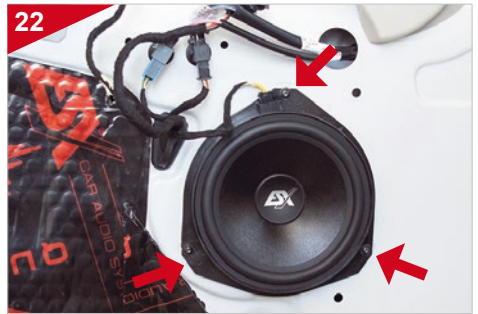
22 Insert the ESX speaker, fasten it with the three original screws and plug in the connector at the top.
