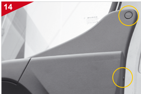
14 Finally, unscrew the screw on the top right of the door panel and the screw underneath on the outside.
