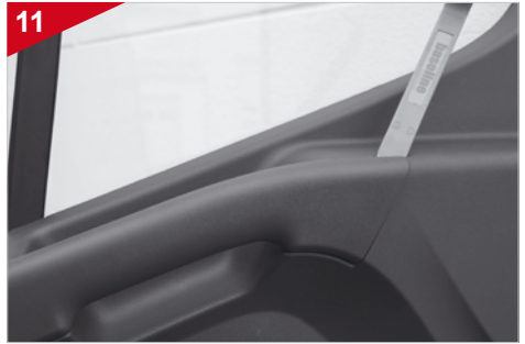
11 Then lever out the door handle with a mounting wedge.
