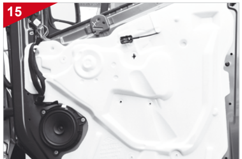
15 You can then unclip the complete door panel from the door and put it aside.
