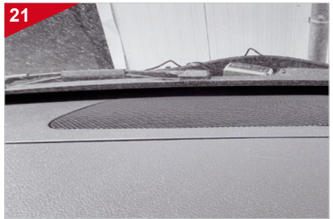
Finally, clip the speaker cover back in and make sure it snaps into place correctly.
