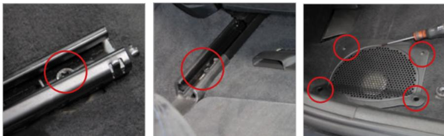
To install the subwoofer, the front seats, which are each fastened with 4 screws, must be removed.
